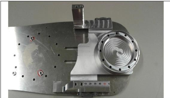
Adjustment mechanism for the length of thigh
