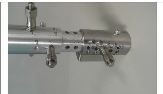
Mechanism for adjusting the length of the lower leg and the angle of the foot plate
