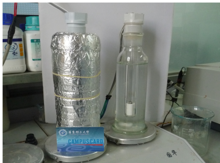
Experimental setup of two 10W UV batch reactors with (left) and without (right) cover.
