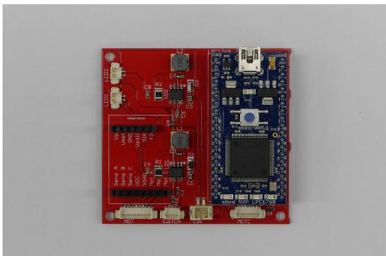
Electronics for the end-effector with mounted microcontroller and embedded driver for the LED's.
