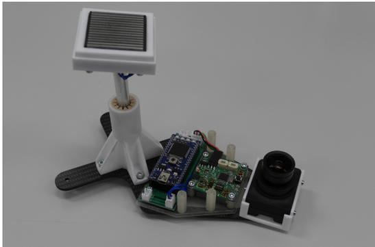
Gripper with electronics and camera mounted on the baseplate.
