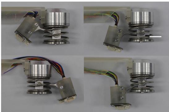
End-effector for tree cavity inspection in four positions through the scan process.
