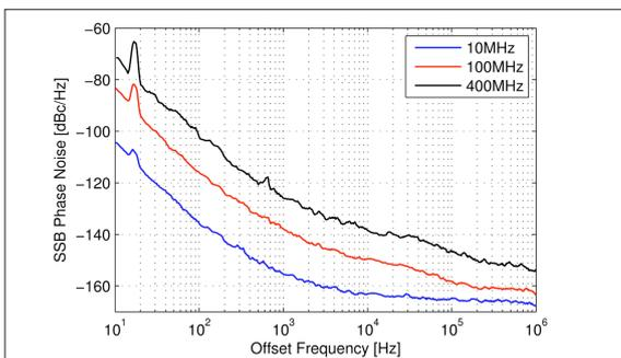
Output phase noise performance at different output frequencies
