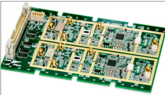
Assembled PCB with two independent reference signal sources
