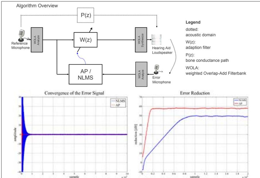
the own speech signal in the canal. Specifically, the LTI System  $P$  in the figure can be estimated with a FIR filter. Two different algorithms were used to estimate the system  $P$ . The figure shows the implemented structure of the NLMS (Normalized Least Mean Square) algorithm and the AP (Affine Projection) algorithm.
