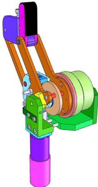
Figure 1: Finger of the Gripper
