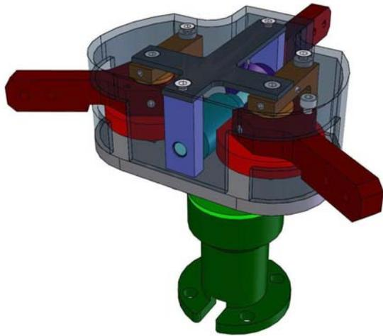
**Figure 2:** Palm of the Gripper
